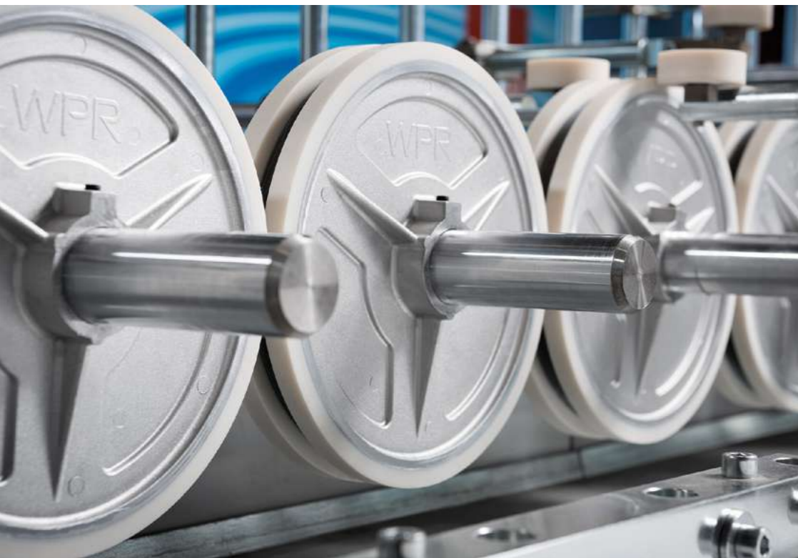
Transport wheels covered in anti-slipping and heat-resistant material
